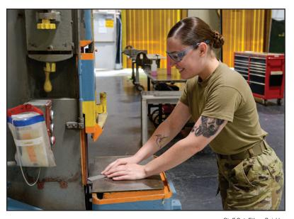
Airman 1st Class Kyleeann Engle, 445th Maintenance Squadron aircraft metals technology technician, shapes metal using a belt sander at Wright- Patterson Air Force Base, Ohio, July 9, 2023. Airmen in Metals Technology use a variety of tools to fabricate and repair metal parts for aircraft and equipment in support of the 445th Airlift Wing mission. The 445th MXS is part of the 445th Airlift Wing, and home to nine C-17 Globemaster III aircraft.
